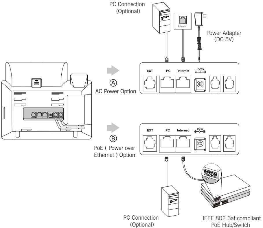
Note: If inline power (PoE) is provided, you don't need to connect the power adapter. Make sure the hub/switch is PoE-compliant.
